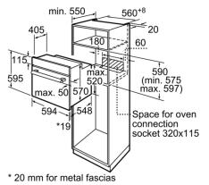
measurements in mm
